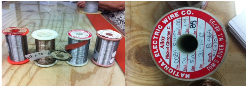
Figure 3: In this figure we show the different material and spools the machine will handle to create the resistance wire.
