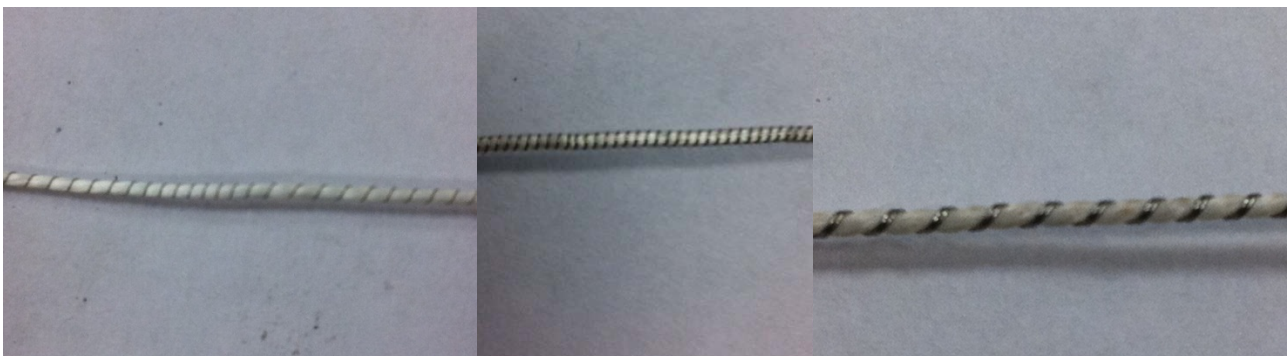
Figure 4: Example of the Heating Resistance Wire. There are different materials used for each and have different resistances due to the loops of wire around the core. Also notice the double wire wind on the right
